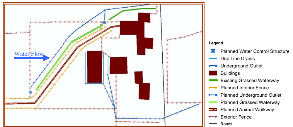
Plan view of the storm water management practices installed at the farm.
